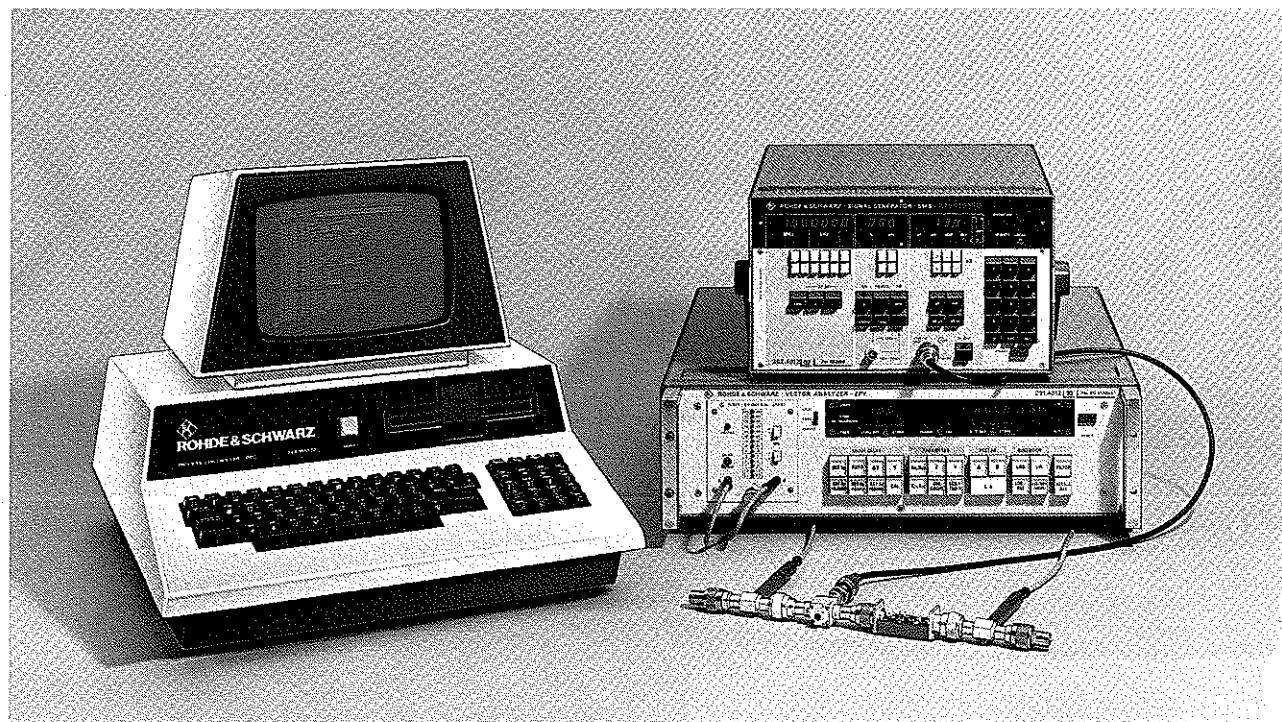
The Signal Generator SMS being used together with the Vector Analyzer ZPV and the Process Controller PPC in a computer-controlled test assembly for s-parameter measurement.
